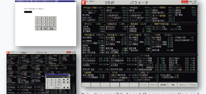
It is also possible to set the pre-purge time and the cutting temperature of the pilot burner.
